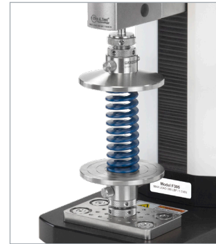
Compression spring testing
