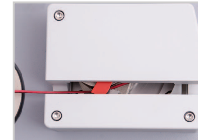
^As the test begins, serrated cams engage the sample. A pinch guard (red tab shown above) automatically rotates into position, for added safety.
